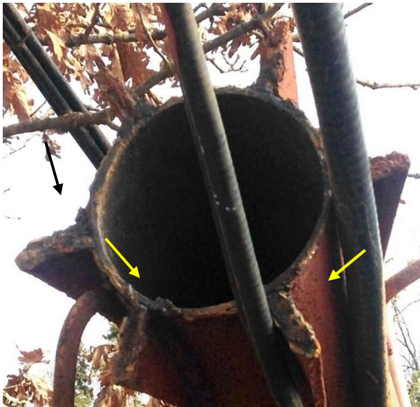
Fig. 4. The critical section at the welded joint
